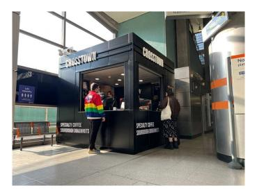
TfL's new station kiosks cut their emissions by 25% by replacing steel with lower-carbon aluminium and using resources more efficiently. Following a successful trial at Shoreditch, the new kiosks are being rolled out across the transport network.
