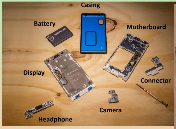
7 different elements in Fairphone's device with an easy access to repair yourself
